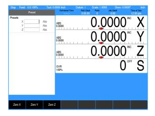
Manually move the table and/or quill until the **INCR** axis positions are zero. When the **INCR** positions are zero, the machine is at the target position.
