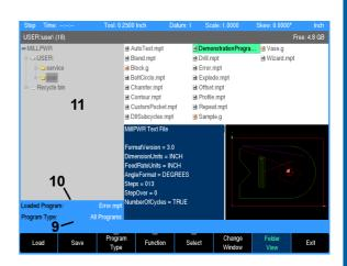
The MILLPWR<sup>G2</sup> can save programs to a USB device, or to network drive (e. g. a PC) as well as to the MILLPWR<sup>G2</sup> User folder.
