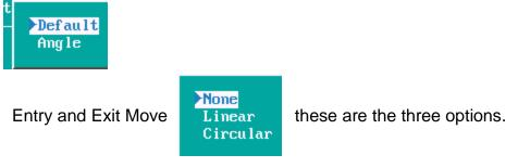
Linear is straight line move on to start point, circular ram on move.
