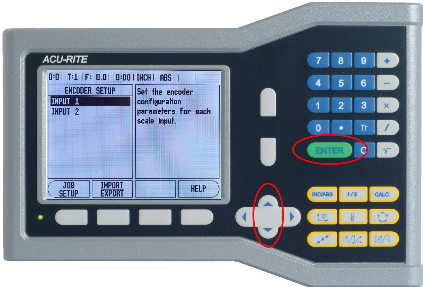
If you need to change more than one axis, highlight the other input axis. Repeat the procedure to change the resolution factor until it matches what is printed on each of the encoders labels. Press **ENTER** after each change to save them.
