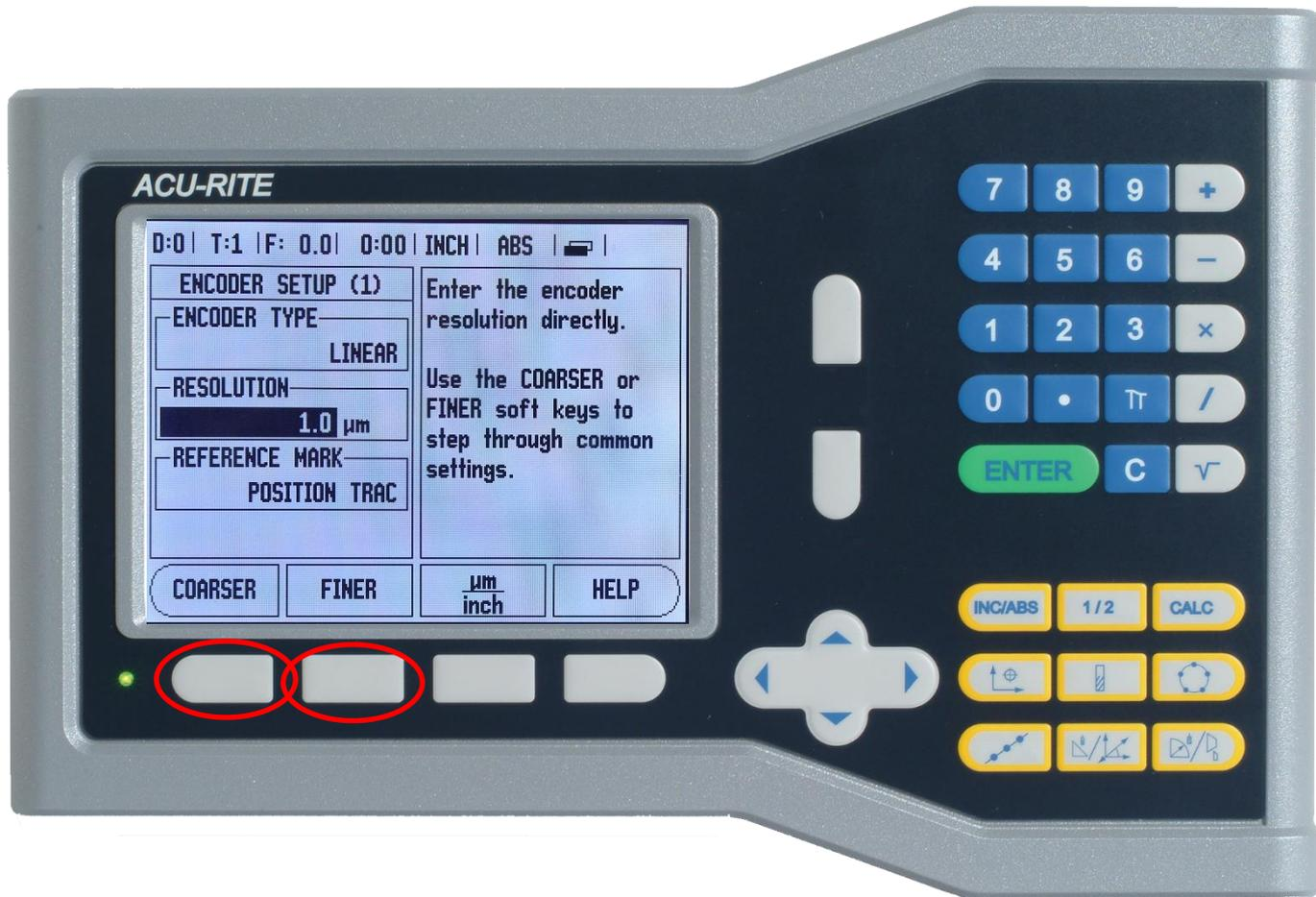
Use the “COARSER” and “FINER” soft keys to change the resolution factor until it matches what is printed on the encoder label. As you saw at the beginning, our scale is 1μm. Press **ENTER** to save your selection.
